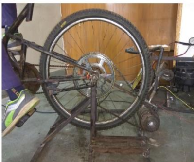
Fig.4 Chain Drive connecting with Compressor
