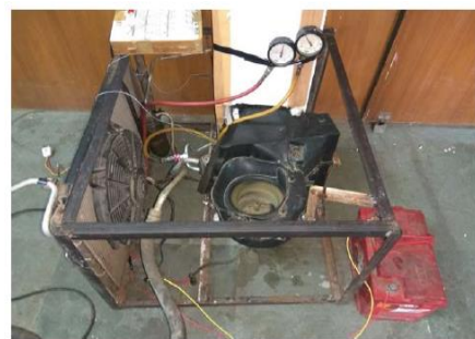
Fig 5: Condenser Fin tube type condenser
