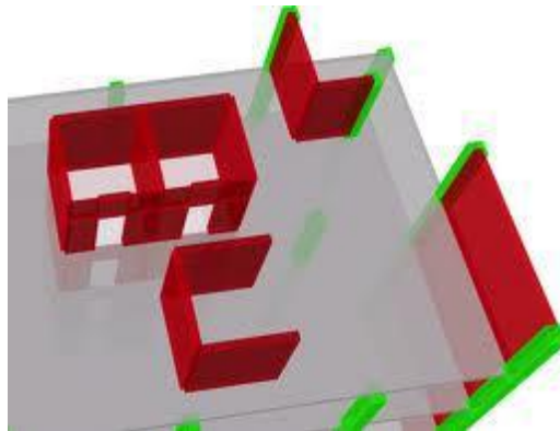
Fig.1 Type of Shear Wall
