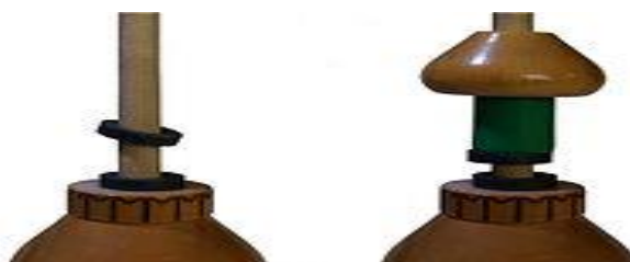
Fig. 11 An example of magnetic levitation with a mechanical support (wooden rod) providing stability.
